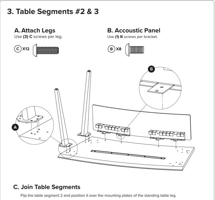
Attach (3) C screws to each leg from underneath the table, connecting the two table segments. If needed, slightly loosen the bolts on the mating legs to ensure proper hole alignment and a snug fit.
