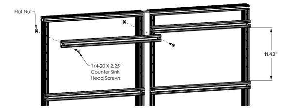
With the top Horizontal Extrusion in place, with a pencil mark the vertical extrusions 11.42" from the bottom of the top horizontal extrusions.
