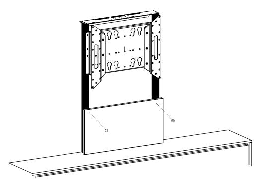
To remove or re-install the Modesty Panel, remove S bolt with the hex key supplied.
