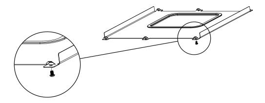
B. Insert plenum into desired bay. Ensure when installing, the mounting tabs sit flush to the bottom surface of the extrusion. Tighten hardware.
