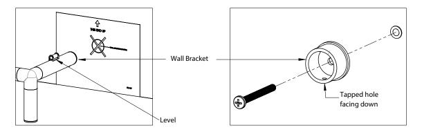
3. Remove the Wall Brackets from the rail and attach to the snaptoggler wall anchor with the Wall Bracket's tapped hole facing straight down, as shown. Repeat on other side.
