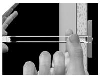
Hold ends of straps between thumb and forefinger and pull toward you until channel rests flush behind wall. Slide plastic cap along straps with either hand with flange of cap is flush with wall.
