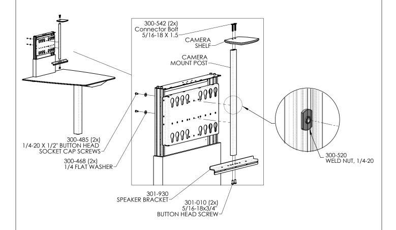
Attach the tech shelf and/or speaker/camera bracket by using the hardware in the locations shown above.
