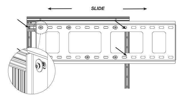
Loosen bolts fastening the horizontal mounting extrusions to vertical mounting extrusions. The flat nuts at the back of the vertical mounting extrusions will drop and need to be repositioned.
