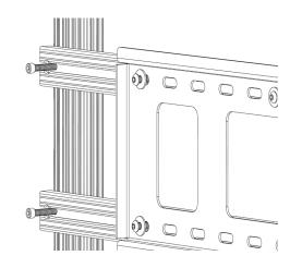
If vertical adjustment are necessary reposition the horizontal mounting extrusions with the fasteners in place and refasten to the vertical mounting extrusions. Level the wall bracket while retightening move to step 2F if horizontal adjustments are needed.
