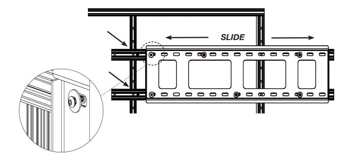
Loosen bolts fastening the horizontal mounting extrusions to vertical mounting extrusions. The flat nuts at the back of the vertical mounting extrusions will drop and need to be repositioned.
