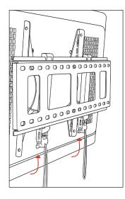
Center TV Brackets on Wall Bracket and push black Click Fasteners up into lock position.
