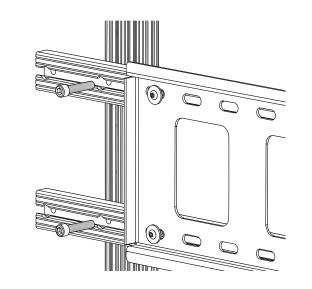
If vertical adjustment are necessary reposition the horizontal mounting extrusions with the fasteners in place and refasten to the vertical mounting extrusions. Level the wall bracket while retightening move to step 4F if horizontal adjustments are needed.
