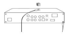
Use supplied magnetic cube to hold thermistor in place on top of the hottest piece of equipment closest to the heat source.
