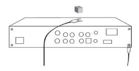
Use supplied magnetic cube to hold thermistor in place on top of the hottest piece of equipment closest to the heat source.
