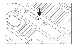
Alternative connection, connect the thermistor directly to the component. Loosen screw and slip the thermistor wire under the screw head and tighten.
