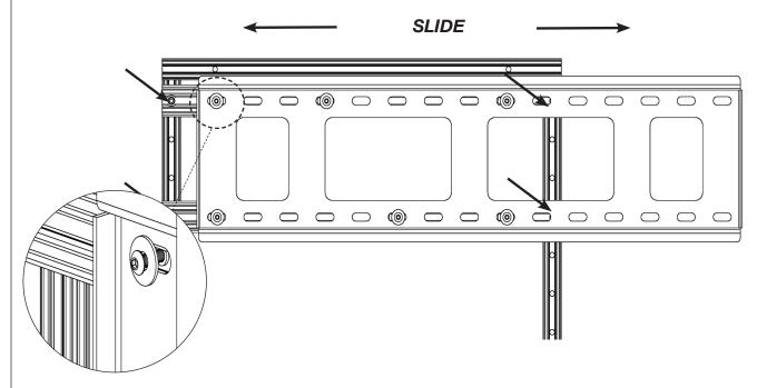
Loosen bolts fastening the horizontal mounting extrusions to vertical mounting extrusions. The flat nuts at the back of the vertical mounting extrusions will drop and need to be repositioned.
