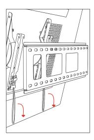
Pull on black cord to unlock Click Fasteners and hook TV Brackets onto Wall Bracket from top.
