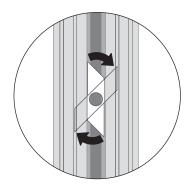
Insert Drop-In Nut (O) into the slots of the vertical mounting post and using the provided Hex Key.
