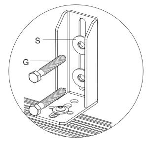
Place cabinet in place and fasten with washers (S) and Lag Bolts (G).
