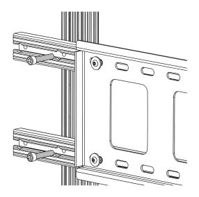
If vertical adjustment are necessary reposition the horizontal mounting extrusions with the fasteners in place and refasten to the vertical mounting extrusions. Level the wall bracket while retightening move to step 4F if horizontal adjustments are needed.
