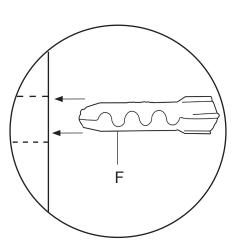
Insert wall anchors (F) into hole.
