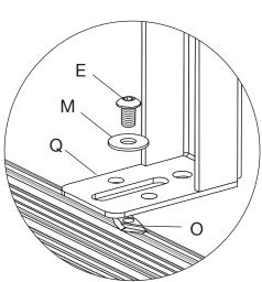
Loosely mount Bracket (Q) using Screw (E), Washer (M) and Drop-In Nut (O).
