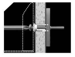
Move cabinet to wall and attach bracket. Insert bolt through Bracket and tighten until snug against wall.
