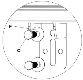
Place cabinet in place and fasten with washers (F) and Lag Bolts (C).
