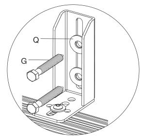
Place cabinet in place and fasten with washers (Q) and Lag Bolts (G).
