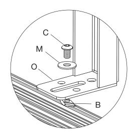
Loosely mount Bracket (O) using Screw (C), Washer (M) and Drop-In Nut (B).
