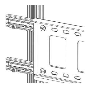
If vertical adjustment are necessary reposition the horizontal mounting extrusions with the fasteners in place and refasten to the vertical mounting extrusions. Level the wall bracket while retightening move to step 2F if horizontal adjustments are needed.
