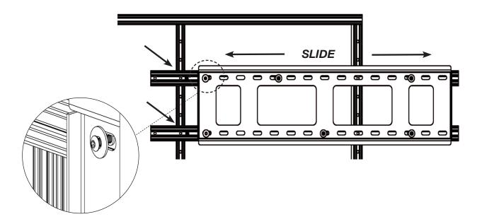
Loosen bolts fastening the horizontal mounting extrusions to vertical mounting extrusions. The flat nuts at the back of the vertical mounting extrusions will drop and need to be repositioned.
