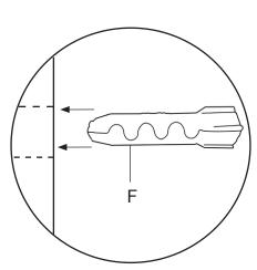
Insert wall anchors (F) into hole.
