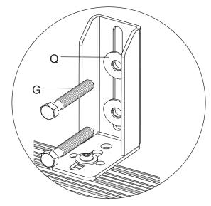
Place cabinet in place and fasten with washers (Q) and Lag Bolts (G).
