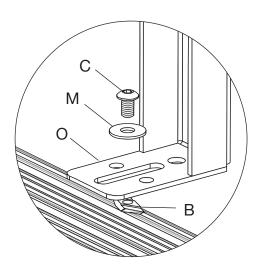
Loosely mount Bracket (O) using Screw (C), Washer (M) and Drop-In Nut (B).
